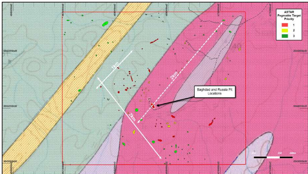
Figure 5: ASTER Pegmatite target zones over geology and inferred strike lengths and widths of the pegmatite occurrences.
